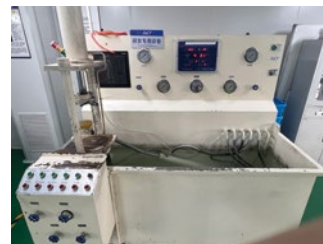
Pressure Test for Large Valve
