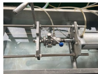
Pressure Test for Small Valve
